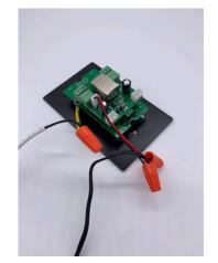
Be sure to ground your SM-8! The SM-8 has a short ground whip attached to the back. This can be grounded to the outlet that is providing power. See image below.
